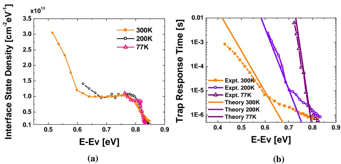
Figure 9 (a) Extracted interface state density versus energy (b) Extracted trap response time versus energy compared to theoretical response time.
