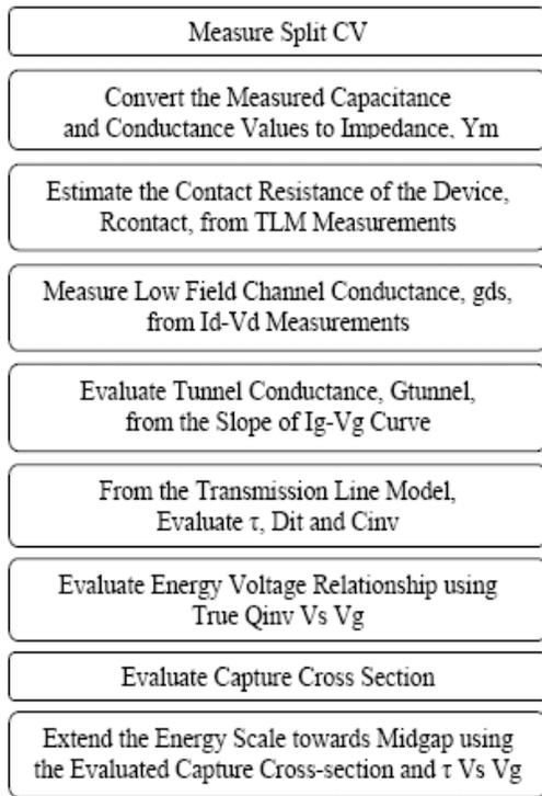
Figure 7 Flow chart of the algorithm used to extract the  $\tau_{it}$ ,  $D_{it}$  and  $N_{inv}$  from the measured CV and GV data in a self consistent fashion.
