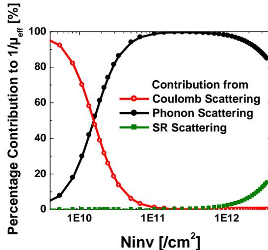
Figure 13 Percentage contributions of Coulomb, Phonon and Surface Roughness (SR) scattering to  $1/\mu_{\text{eff}}$
