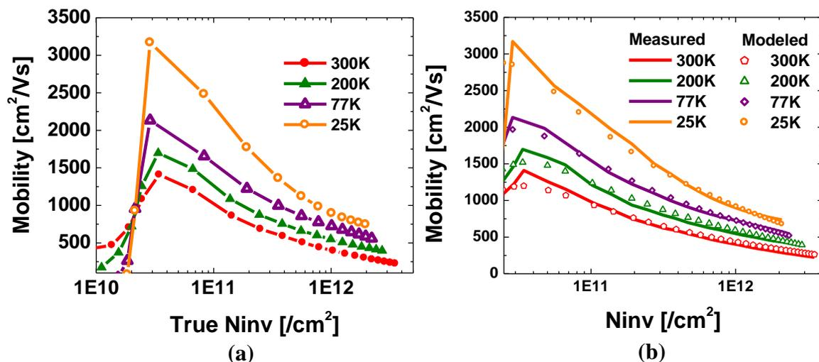
Figure 12(a) Effective mobility as a function of inversion charge (b) Experimental mobility compared with the model
