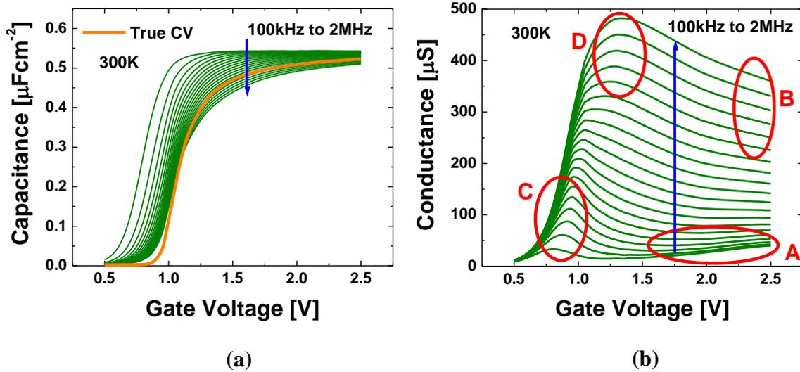
Figure 5 Effect of interface states, series resistance (contact and channel) and tunnel conductance on the (a) measured C-V characteristics and (b) measured G-V characteristics.
