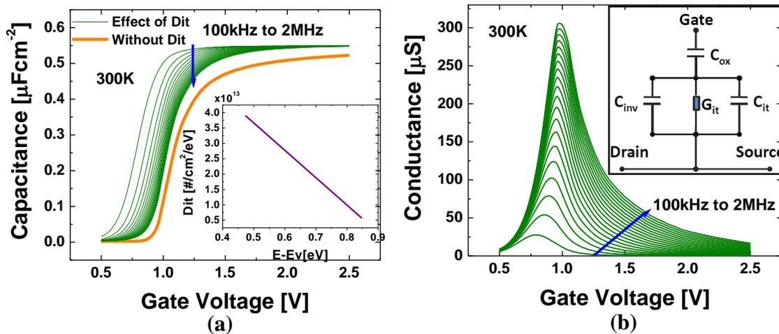
Figure 4 (a) Effect of interface states,  $D_{it}$ , on the measured C-V characteristics (b) Effect of interface states,  $D_{it}$ , on the measured G-V characteristics. The equivalent circuit model in inversion incorporating the effect of  $D_{it}$  is shown in the inset of (b)
