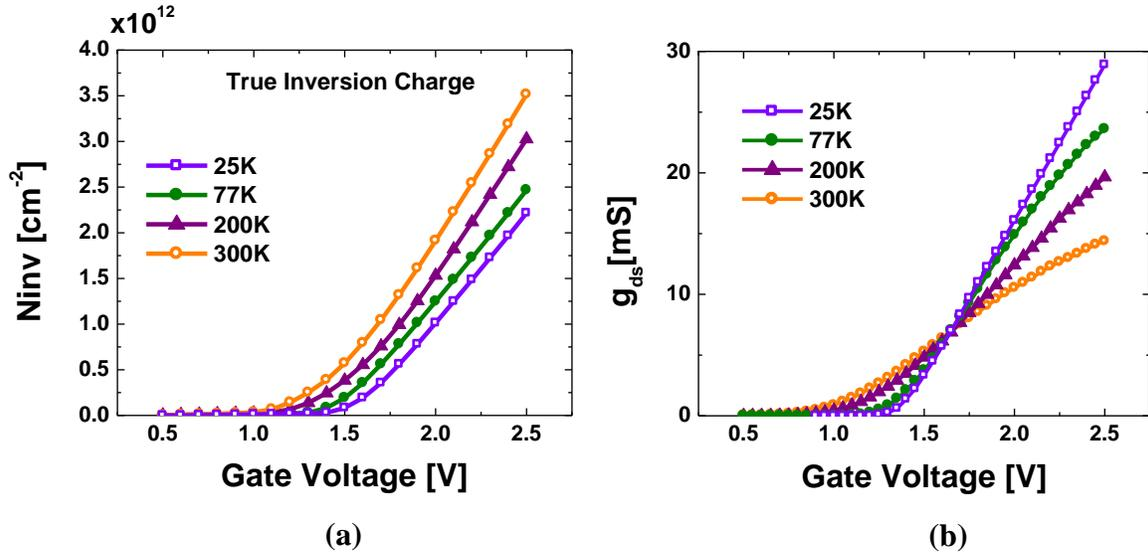
Figure 11 (a) Extracted  $N_{inv}$  from the C-V and G-V measurements and (b) the measured DC channel conductance data at 300K, 200K and 77K
