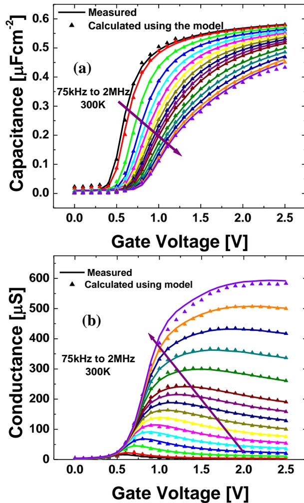
Figure 8(a) Experimental CV and (b) Experimental GV compared to solution from the split CV model
