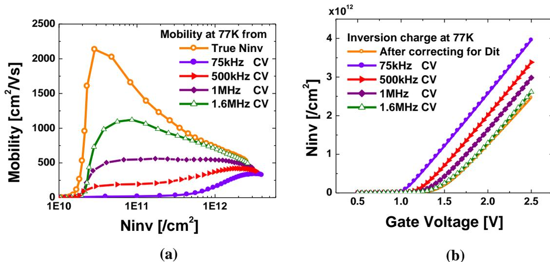
Figure 1 Comparison of (a) effective channel mobility and (b) inversion carrier density at 77K with and without correction for interface states, gate leakage and distributed channel resistance
