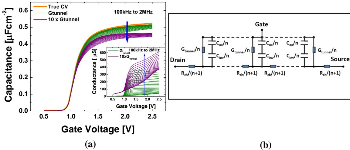
Figure 3 (a) Effect of tunnel conductance due to gate to channel leakage on the measured C-V and G-V characteristics (b) Equivalent circuit of a MOSFET in inversion incorporating the tunnel conductance, the distributed channel resistance and the contact resistance at each end of the channel.
