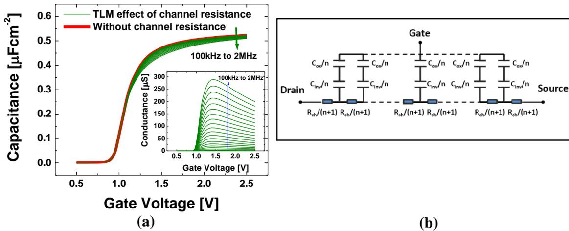
Figure 2 (a) Effect of distributed channel resistance on the measured C-V and G-V characteristics (b) Equivalent circuit of a MOSFET in inversion incorporating the channel resistance and ignoring the effects of interface states and gate leakage.
