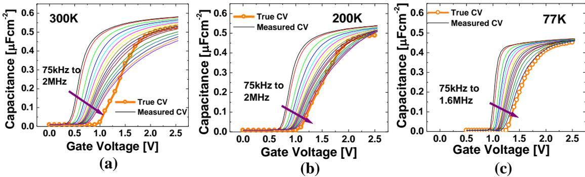
Figure 10 Measured C-V and extracted true C-V characteristics from  $\text{In}_{0.53}\text{Ga}_{0.47}\text{As}$  MOSFETs at (a) 300K (b) 200K and (c) 77K
